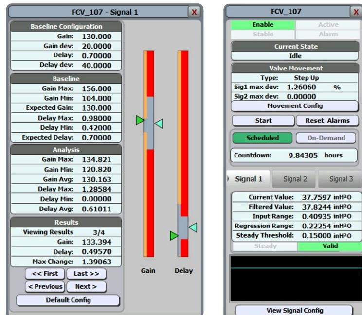
With automated scheduling at desired intervals, the Valve Exerciser makes it easier than ever to continually ensure the health of the critical valves surrounding your compressor.
